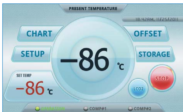
7" Full Touch Screen TFT LCD(Smart-Lab™ Controller)
